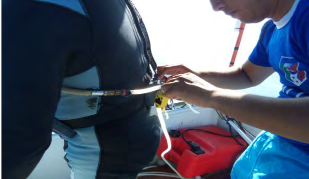
Figure 5. Each consenting fisherman wears a Sensus Ultra dive recorder on his dive belt throughout each dive. The dive recorder is set to collect pressure every 10 seconds, with an accuracy of \pm 1 foot of sea water. This input coupled with a user written algorithm has allowed us to clarify the level of decompression stress these fishermen divers expose themselves to.
